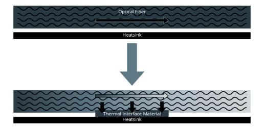
Optical fiber with a high intensity light increases the temperature and can damage the system. Efficient transfer of the heat into a heatsink or structural component at key points along the fiber can significantly reduce risk of failure and improve performance.
